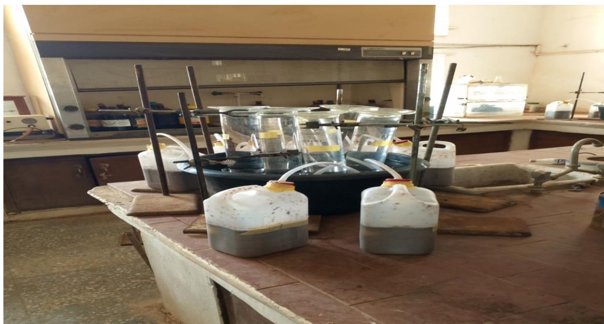
Plate 1: Set up for biogas production from co-digestion of broiler litter and cassava peel
