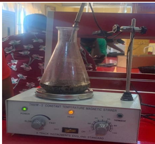
Plate 3: Transesterification Process of Biolubricant after Washing
