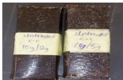
Plate 2: Composites produced from cocoa shell powder and polypropylene
