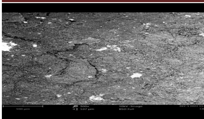
Fig 3(a): SEM micrographs of CA Ag NP
