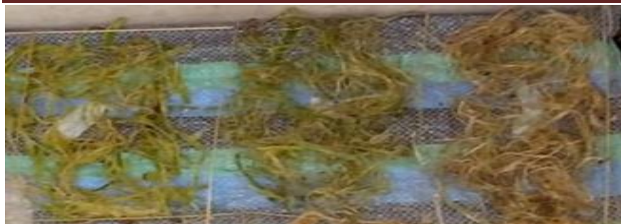
Plate 4: Extracted fibre at different concentrations of HCl
