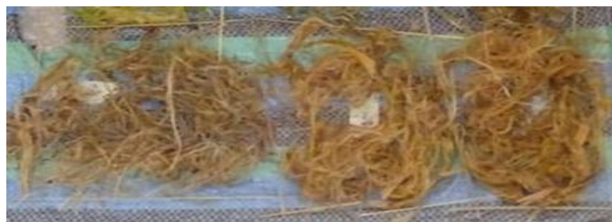
Plate 3: Extracted fibre at different concentrations of NaOH
