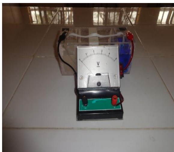
Plate 2: Experimental set up with the constructed voltaic cell
