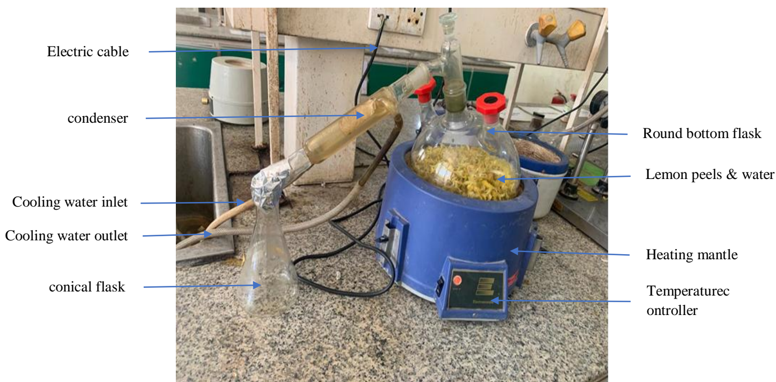
Figure 1: Hydro-distillation set-up for lemon peels extraction of essential oil
