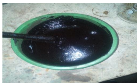
Plate 3: Carbonized bovine horns impregnated with NaOH while stirring
