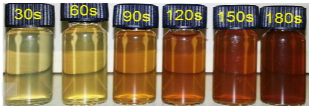
Plate 1: Colour change of reduced silver metal in synthesis of AgNPs at different time intervals from 30 s, 60 s, 90 s, 120 s, 150 s and 180 s.
