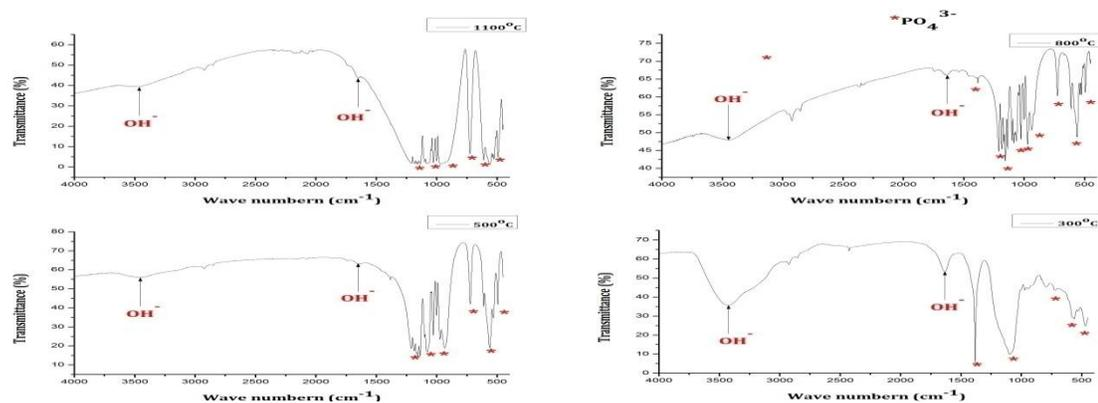
Fig. 8: FTIR spectra of HA synthesized using initial precursor concentration of 2.0M, calcinated at different temperatures.
