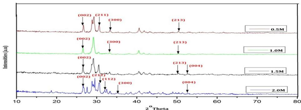
Fig. 10: XRD pattern of HA synthesized via WT method using different initial precursor concentrations and calcinated at 500°C.
