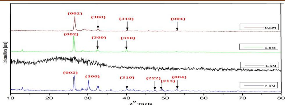
Fig. 9: XRD pattern of HA synthesized via WT method using different initial precursor Concentrations and calcinated at 300°C.
