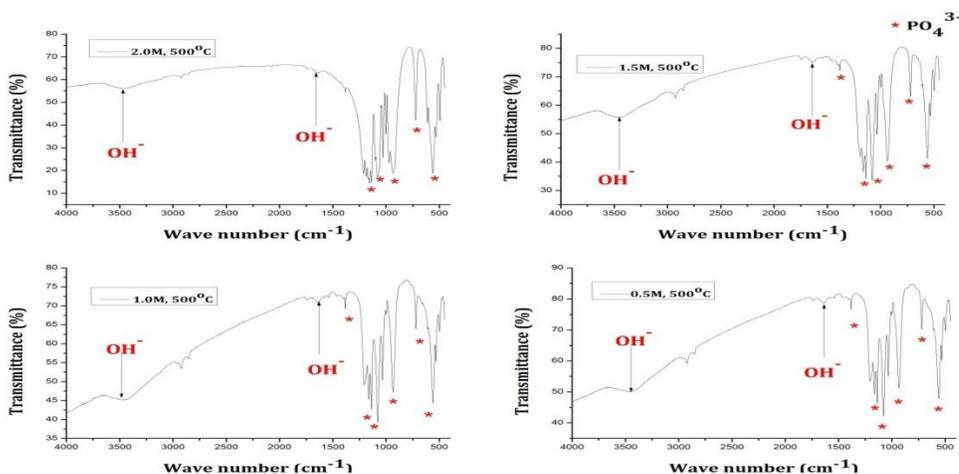
Fig. 2: FTIR spectra of HA synthesized via WT method using different initial precursor concentrations, calcinated at 500°C.
