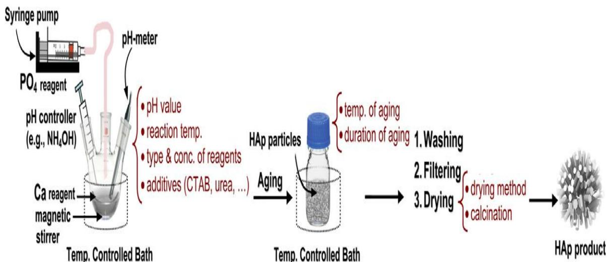
**Scheme 3.2:** Preparation of HA nanoparticles via conventional chemical precipitation
