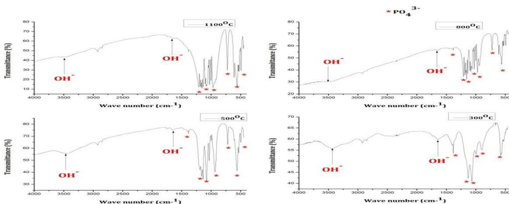
Fig. 7: FTIR spectra of HA synthesized using initial precursor concentration of 1.5M, calcinated at different temperatures.
