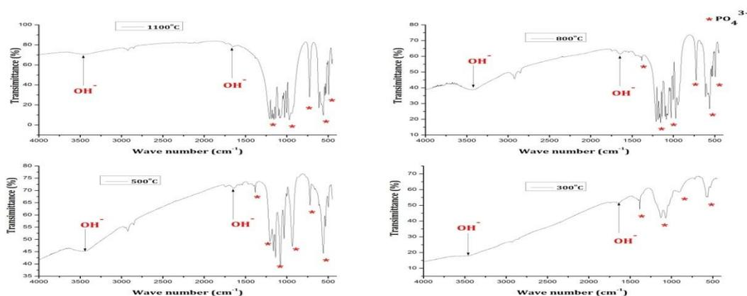
Fig. 6: FTIR spectra of HA synthesized using initial precursor concentration of 1.0M, calcinated at different temperatures.
