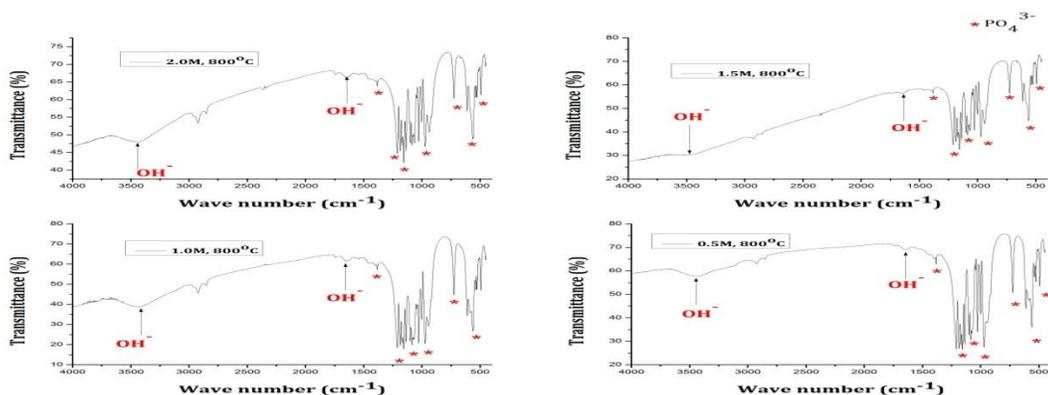
Fig. 3: FTIR spectra of HA synthesized via WT method using different initial precursor concentrations, calcinated at 800°C.
