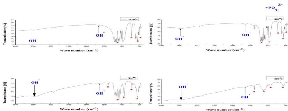
Fig. 5: FTIR spectra of HA synthesized using initial precursor concentration of 0.5M, calcinated at different temperatures.
