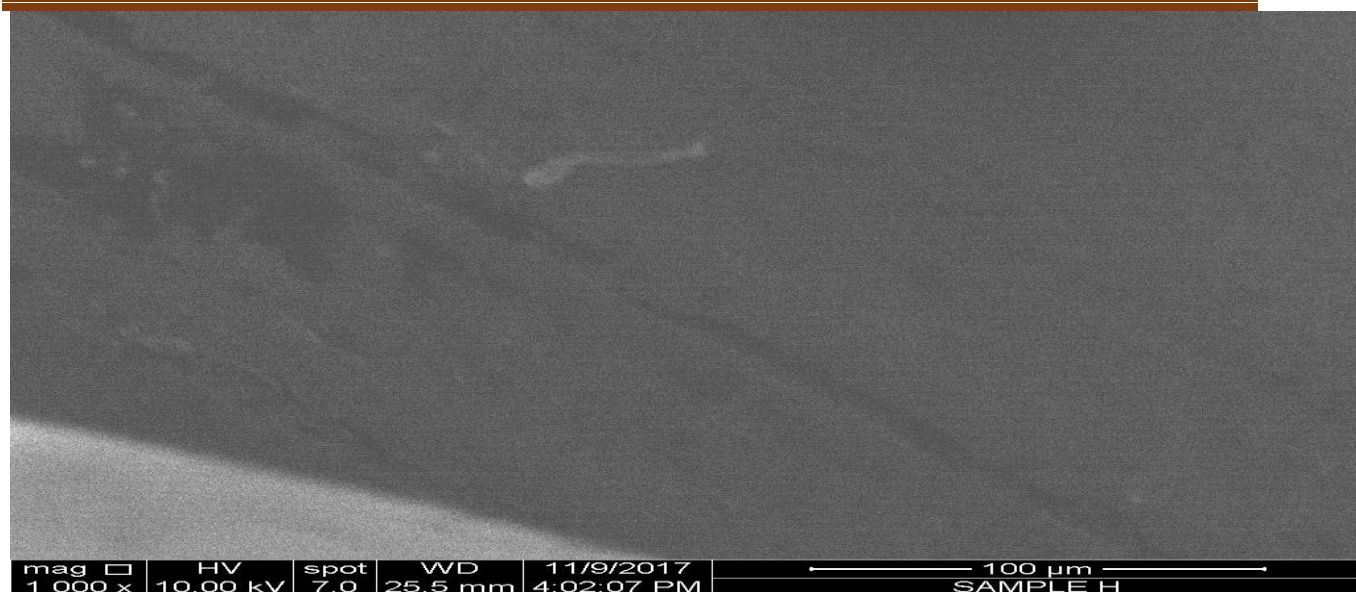
Figure 3.3: Surface Morphology of Unfilled Natural Rubber Vulcanizate
