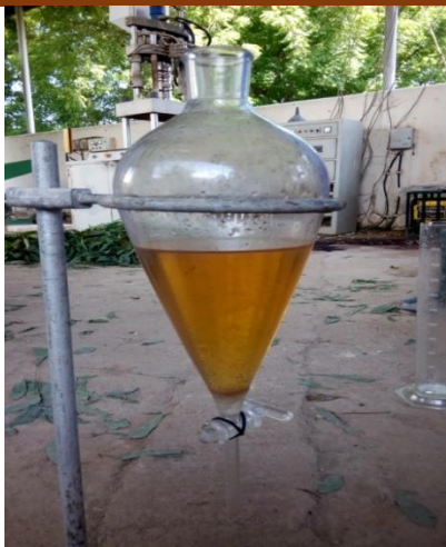
Figure 3: Separating process of essential oil and water
