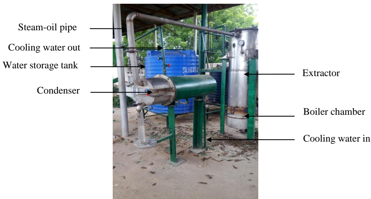
Figure 2: Essential oil extraction pilot plant set-up
