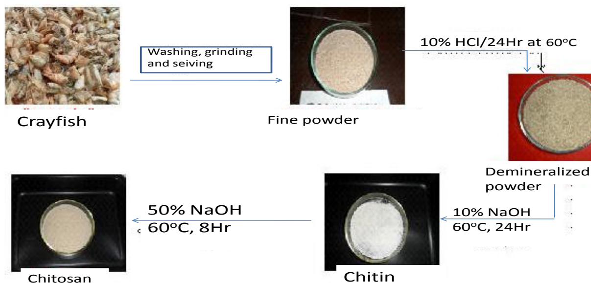
Schematic diagram of chitosan synthesis from crayfish
