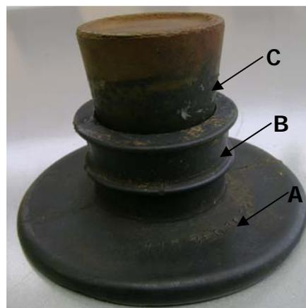
**Figure 1: Showing the fabricated rumen fistula using a car driving shaft cover. The rubber bung is also shown. A, Fistula flange. B, projected end of the fistula. C, rubber bung stoppered on the fistula opening for firm closure**
