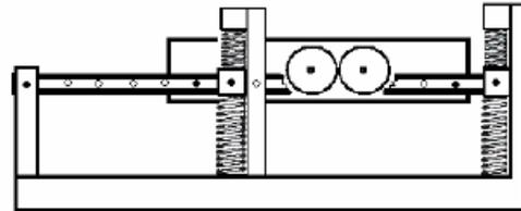
**Figure 1: Vibration simulation device**
