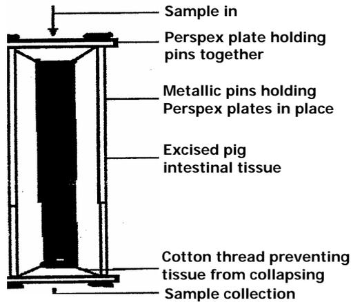
Figure 1: Device for suppository drainage/adhesion experiments
