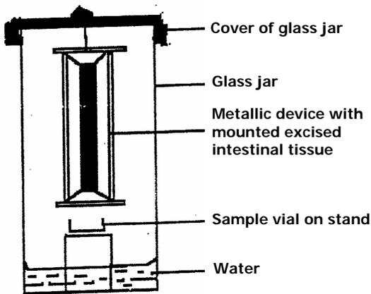
Figure 2: High humidity chamber for drainage experiments
