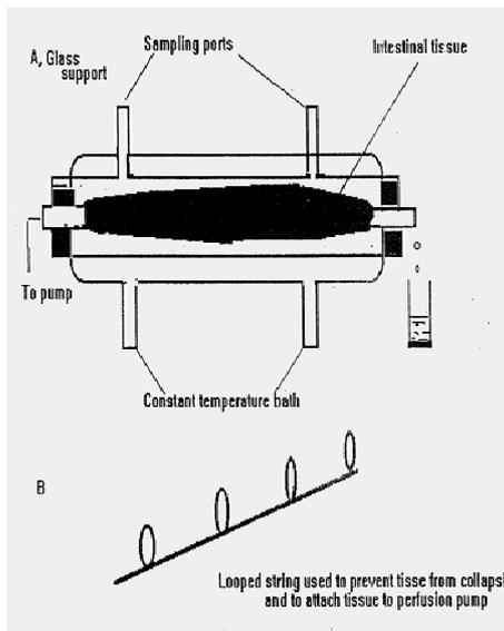
Figure 3: Water-jacketed support for *in-vitro* detachment experiments
