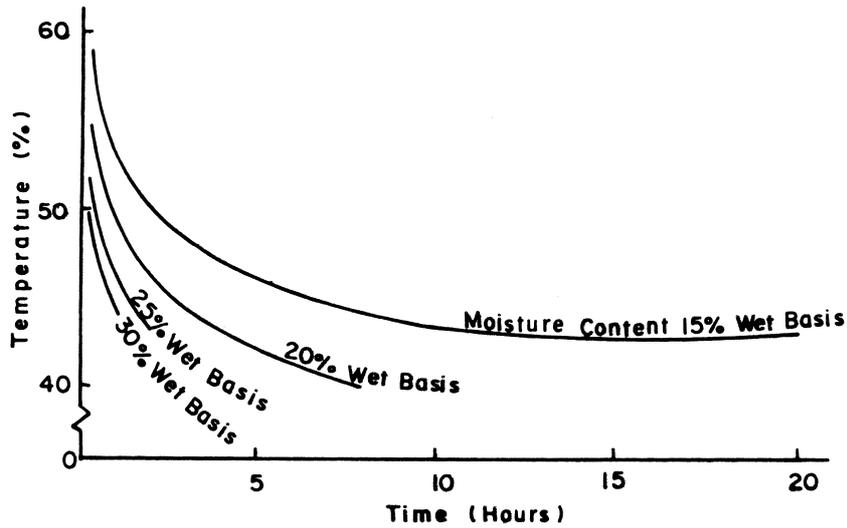
Fig. 4. Maximum heating time for grain at different temperatures and moisture contents in order not to destroy grain viability.
