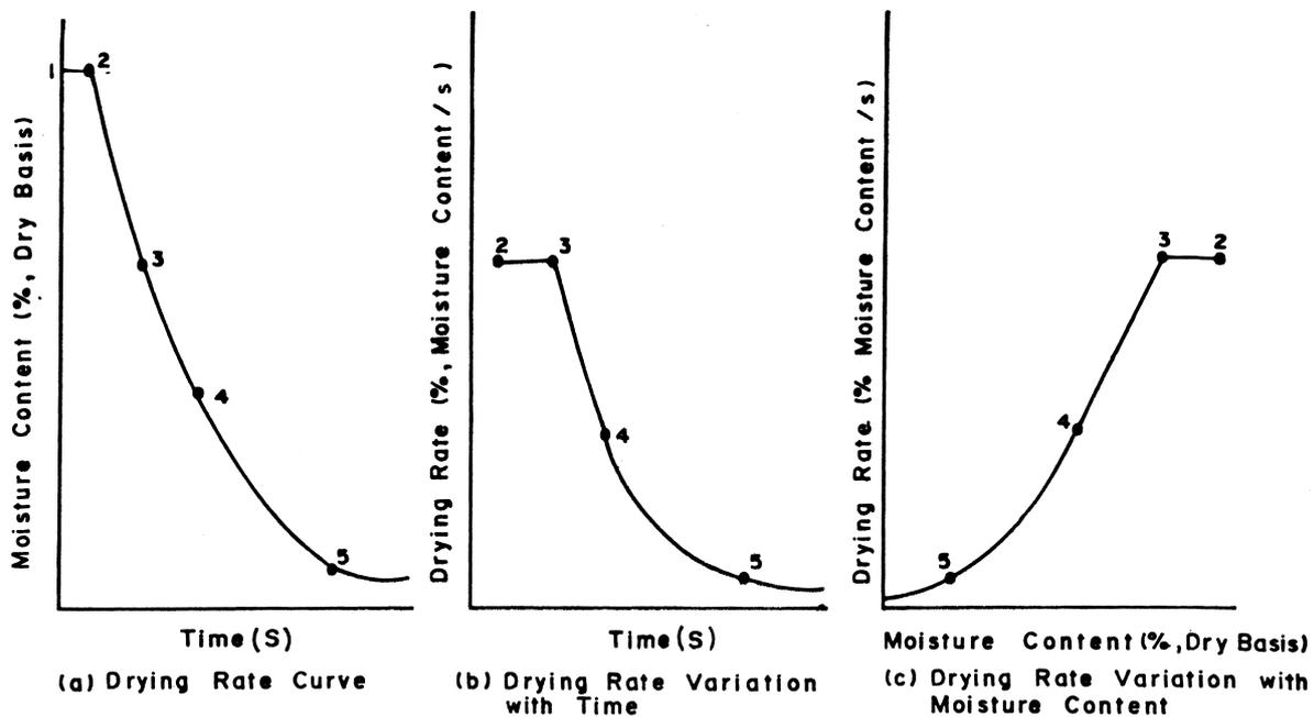
Fig. 7. Schematic illustration of drying rate periods: 1–2 the heating period (constant moisture content); 2–3 the constant rate drying period; 3 the critical moisture content; 3–4 the first falling rate period; 4–5 the second falling rate period.
