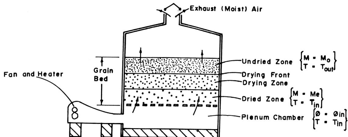
Fig. 8. Schematic illustration of deep bed drying.
