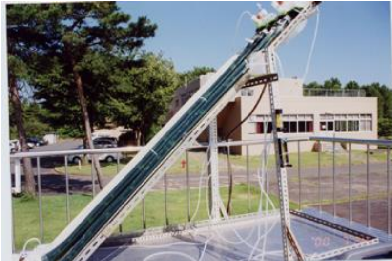
Figure 8. Photograph of tubular photobioreactor with static mixers for improved mass transfer.
