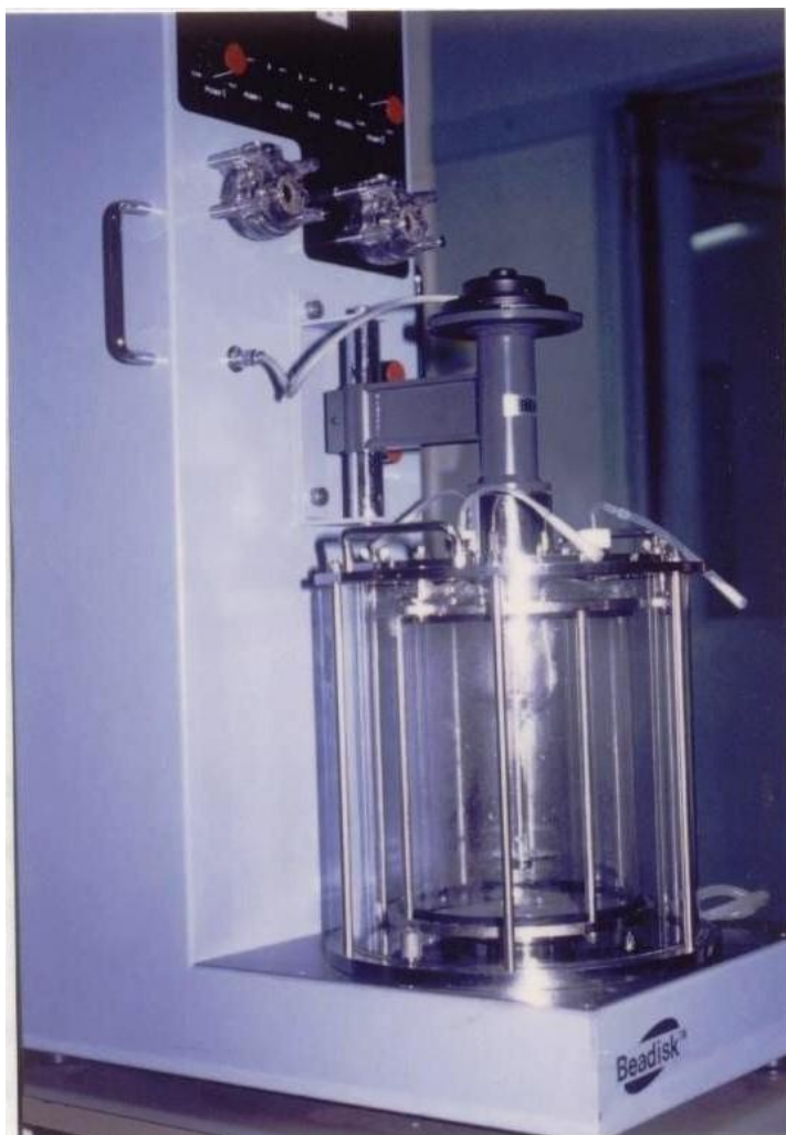
Figure 2. A photograph of the rotating disk atomizer for immobilization of cells in micro-gel beads. This was patented and is now commercially produced by Marubishi Bio-engineering, Japan.
