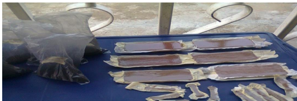
Figure 3: Cast samples of unsaturated polyester/snail shell composite
