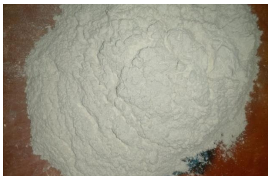
Figure 2: Powder Snail shell after grinding and sieving [13]
