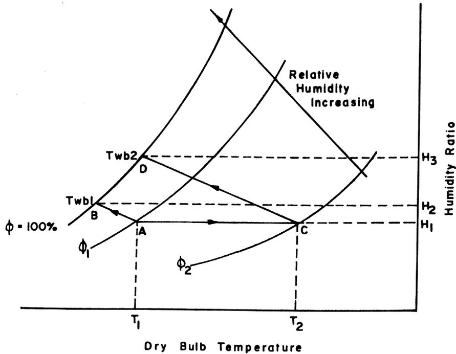
Fig. 10. Schematic illustration of the psychrometrics of drying process.
