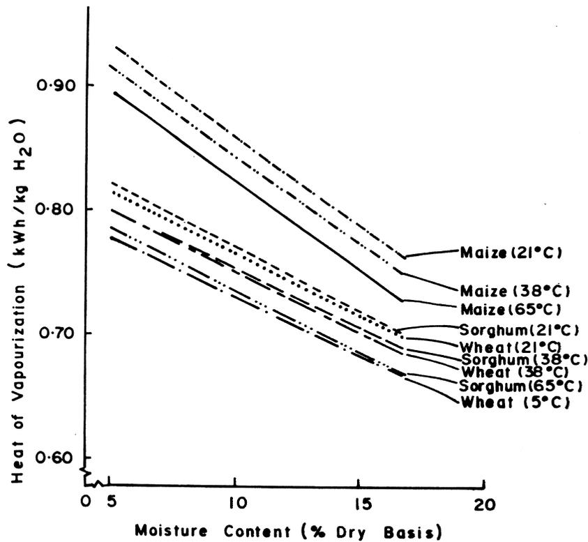
Fig. 2. The variation of heat of vaporization of types of grain with moisture content and temperature.
