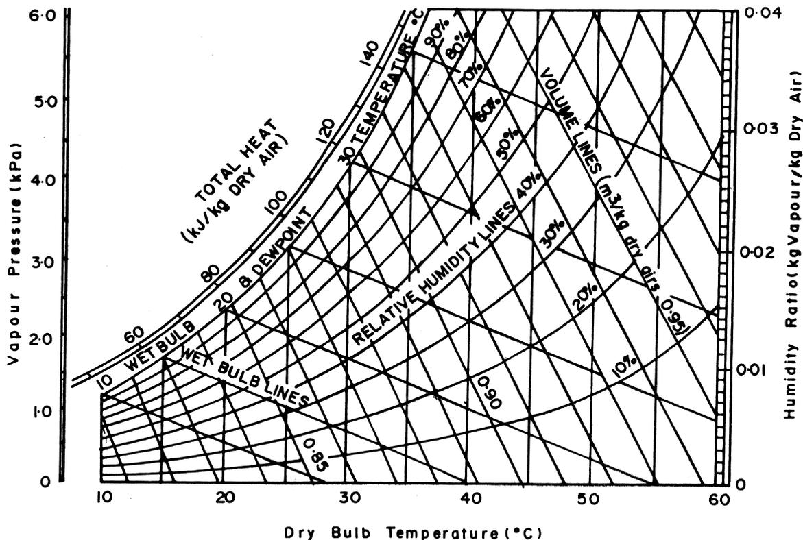
Fig. 9. Psychrometric chart for barometric pressure of 101.325 kPa.
