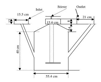
Figure 1. Schematic diagram of the biodigester.
