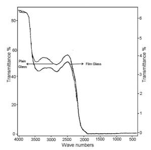
Fig. 1. Spectral infrared transmittance of plain glass and combined film-glass system of a MgCdS<sub>2</sub> sample.
