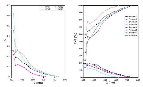
Fig. 2 (left). Spectral absorbance of MgCdS<sub>2</sub> films.
