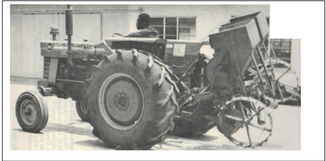
Fig. 3. Automatic cassava planter Model III, (a)— Single-row prototype built in 1981 (b)— Prototype mounted in transport mode 22
