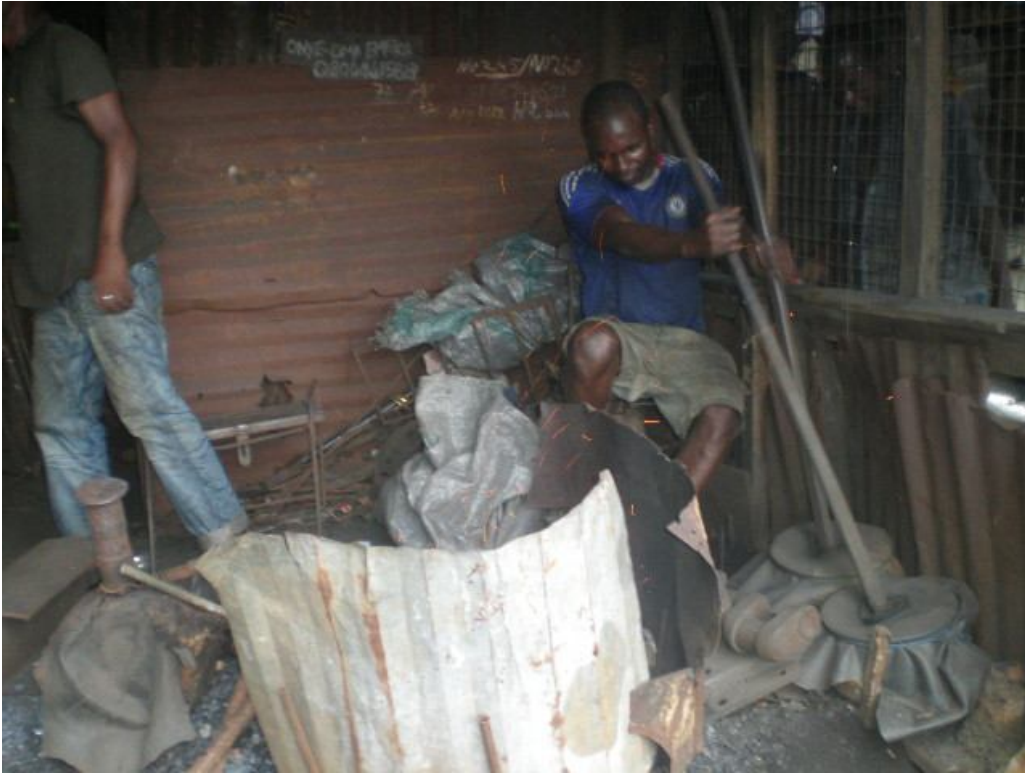
Fig 3: Firing charcoal to melt the brown sand(iron ore) using bellows 21 st century in Nigeria. The environment belongs to the 17 th century period.
