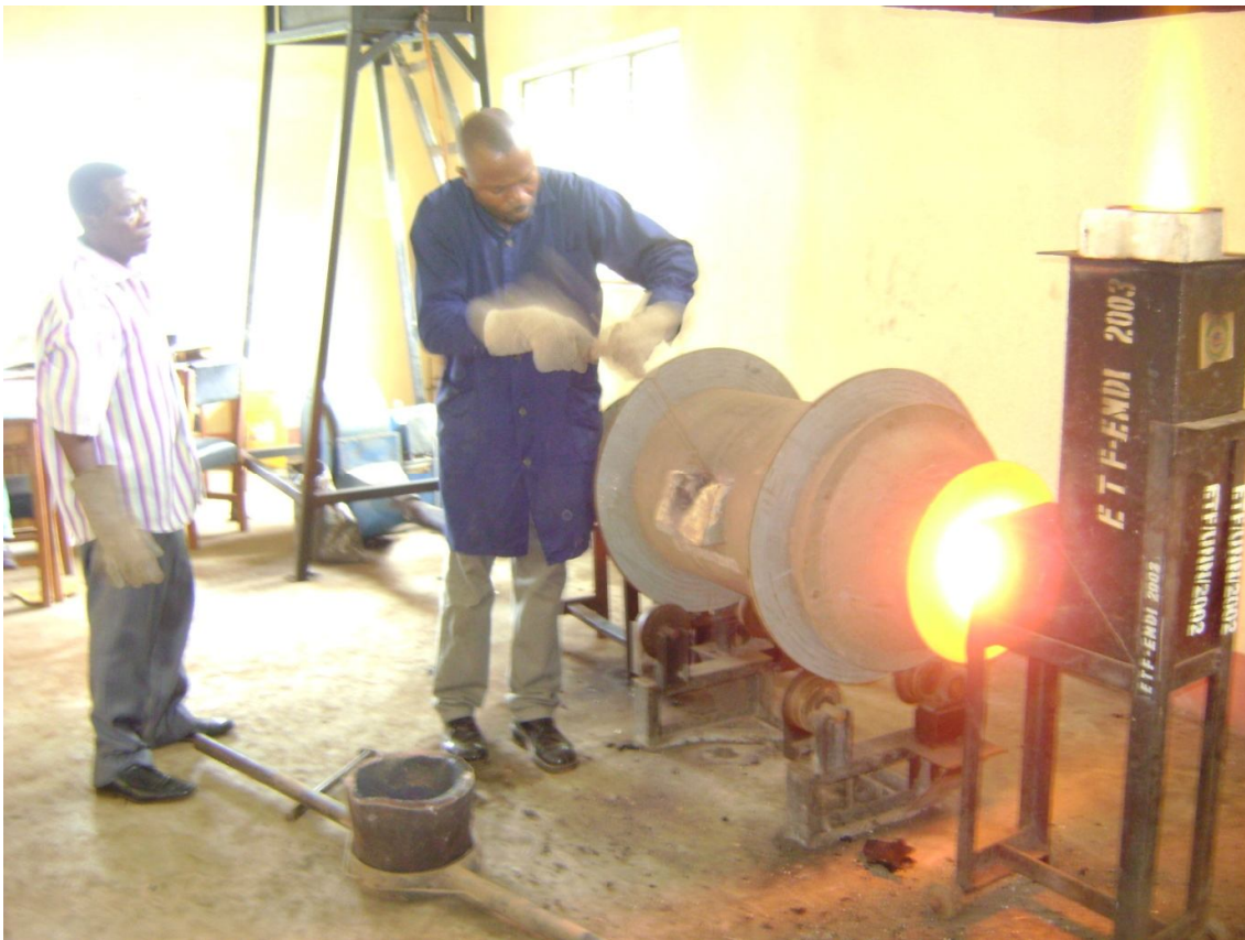
Fig 33: ROTARY FURNACE INSTALLED IN THE FACULTY OF ENGINEERING (Obikwelu et al 2007)
