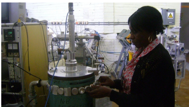
Fig. 10: The inaugural Lecturer determining film composition at iThemba Labs, Cape Town, South Africa using Rutherford Back Scattering, RBS technique. Sept., 2013
